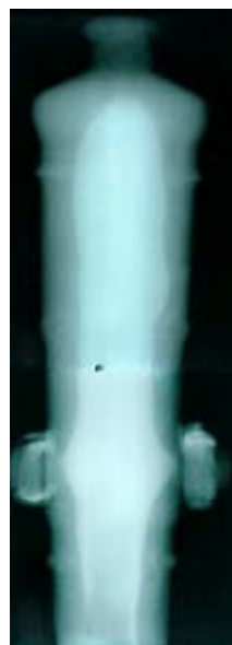
X-ray of a half-pounder swivel gun.
